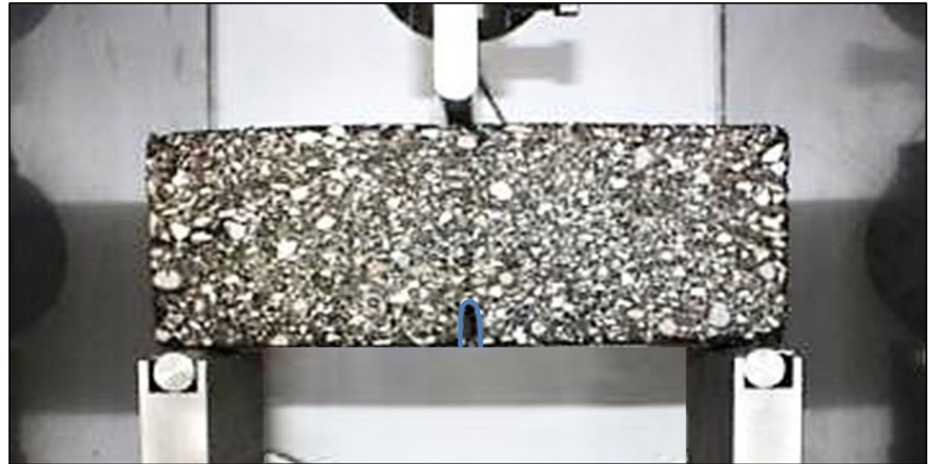
Testing strength of small granite block
